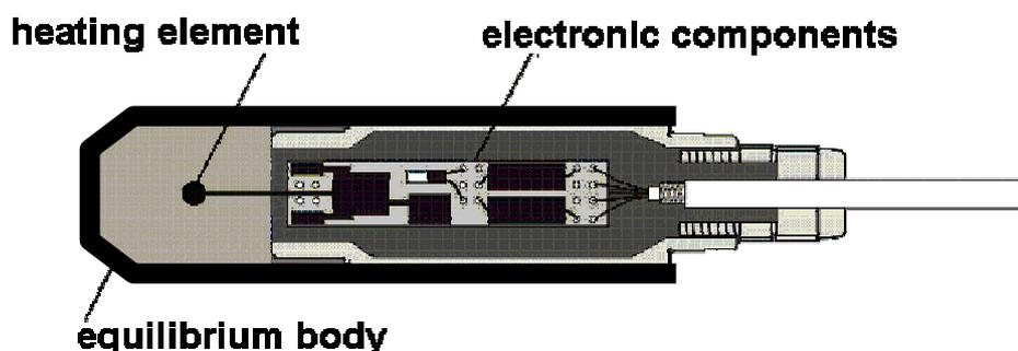
Fig. 2: Structure of the Tensiomark
