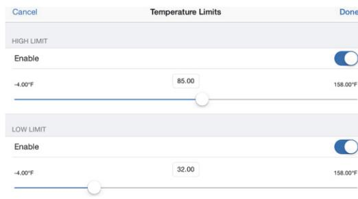
7. Enable Low Limit if you want burst logging to occur when the sensor reading falls below a specific reading. Drag the slider to the reading that will trigger burst logging or tap the value field and type a specific reading. In the example, the logger will switch to burst logging when the water temperature falls below 32°F.
