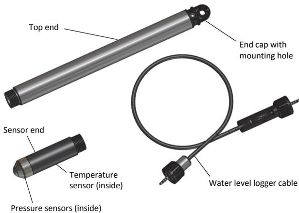
The MX water level logger consists of a top end and a sensor end that is connected by a water level logger cable. The three components work together to allow for wireless transfer of data to the HOBOMobile app on a mobile phone or tablet. This is an overview of each component:
