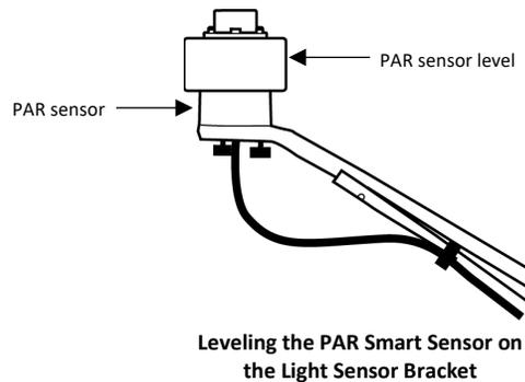
Leveling the PAR Smart Sensor on the Light Sensor Bracket
