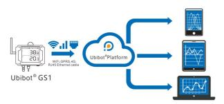
The GS1 continuously monitors environmental conditions and syncs the data to the UbiBot<sup>®</sup>IoT Platform. By offering 4 ways of data transmission, it can ensure different users access the online data using our App or the website.
