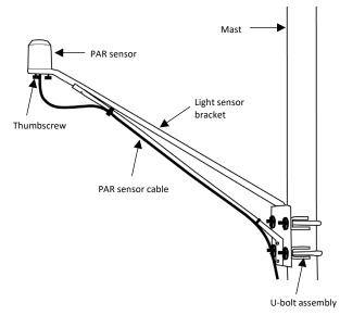
PAR Smart Sensor Bracket Mounting
